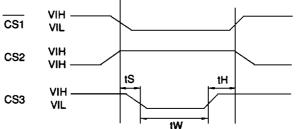
$t_S = t_H = 1 \mu sec (min.)$   $t_W = 10 msec (min.)$  $V_H = 12 \pm 0.5 V$
